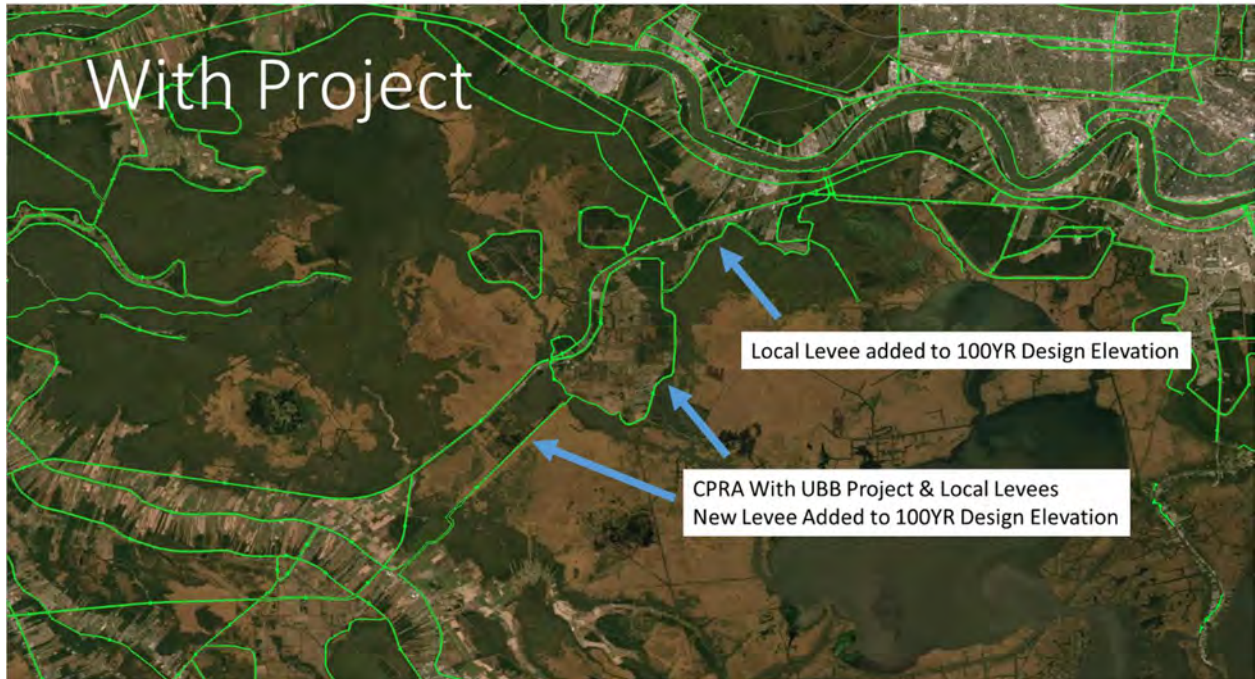
Figure 3 With project - levees and raised feature alignments
